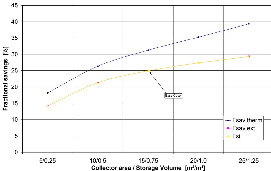
Figure 4. Variation of fractional energy savings with collector size with a fixed specific store volume of 0.05 m<sup>3</sup>/m<sup>2</sup>.
