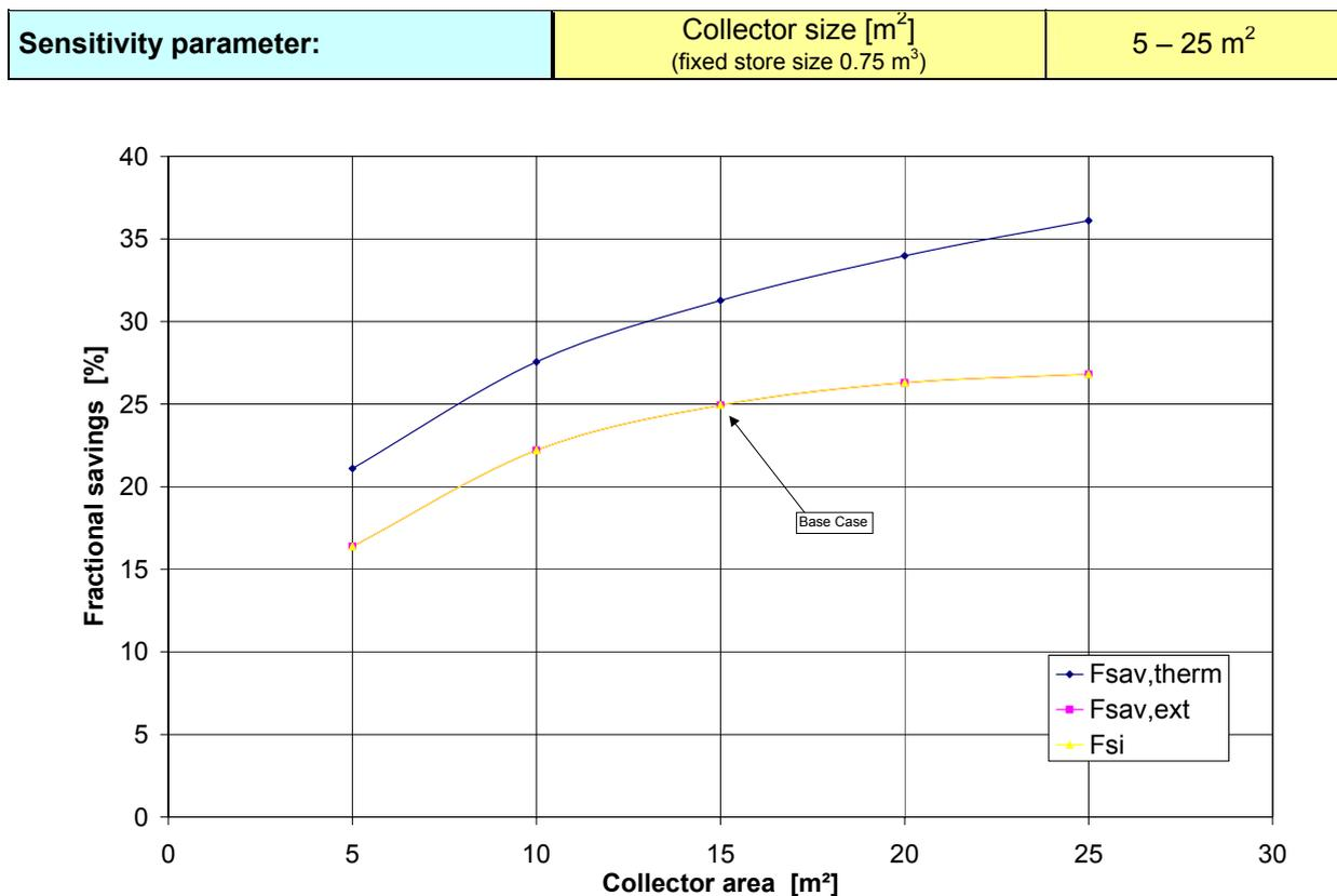
Figure 3. Variation of fractional energy savings with collector size with fixed store volume of 0.75 m<sup>3</sup>.
