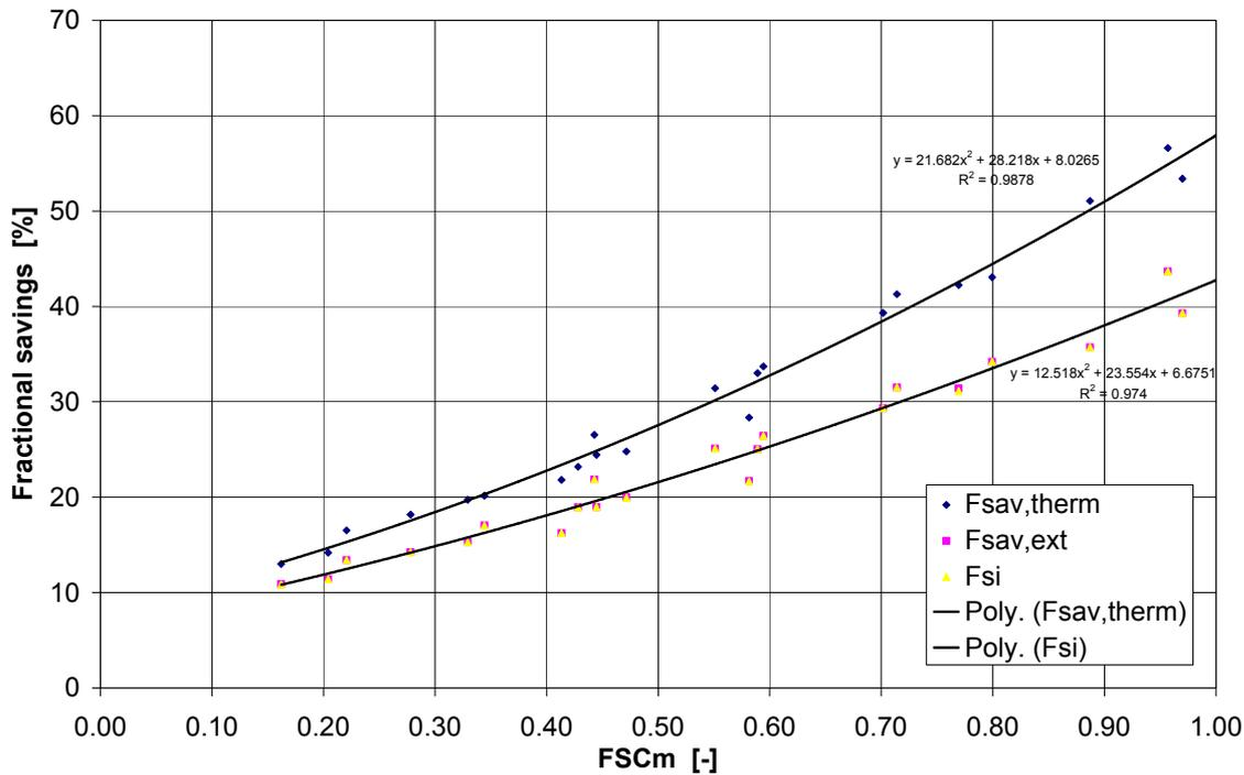
Figure 22: Fractional savings for the base case combisystem as a function of the FSC-value for 3 climates (Carpentras, Zurich, Stockholm) and 3 loads (30, 60, 100 kWh/m<sup>2</sup>a single family buildings).
