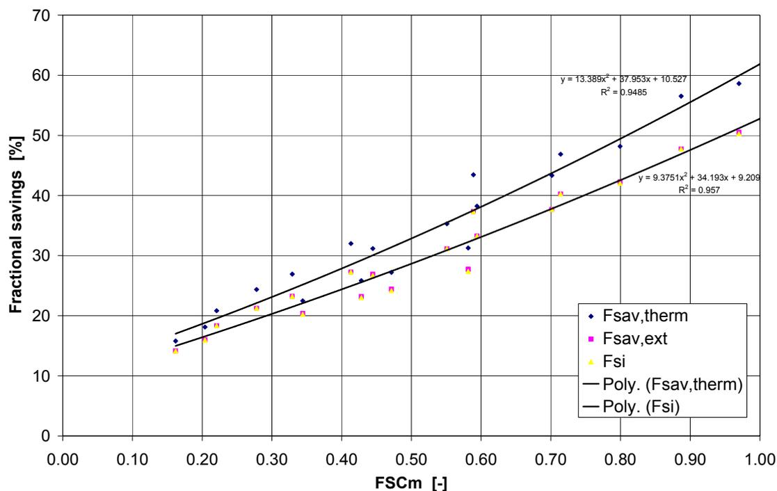
Figure 23: Fractional savings for the improved combisystem as a function of the FSC-value for 3 climates (Carpentras, Zurich, Stockholm) and 3 loads (30, 60, 100 kWh/m<sup>2</sup>a single family buildings), Improved system.
