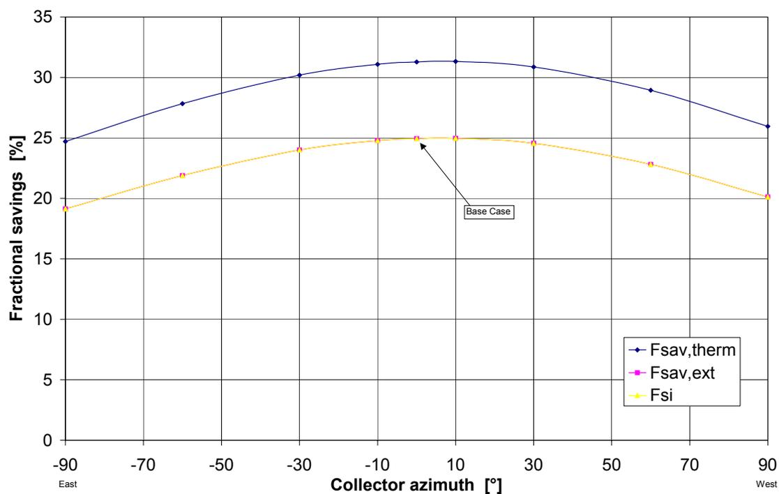
Figure 6. Variation of fractional energy savings with collector azimuth with fixed tilt angle of 45°.
