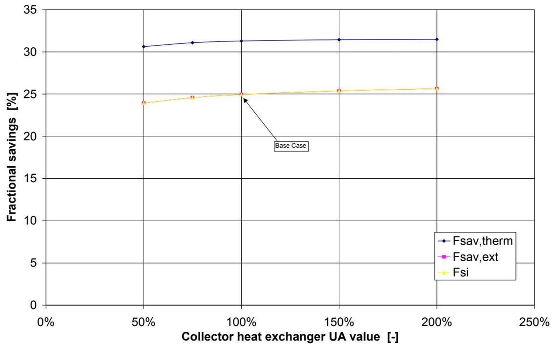
Figure 9. Variation of fractional energy savings with the UA-value of the collector heat exchanger. Parameter values are relative to the values defined for the base case system.
