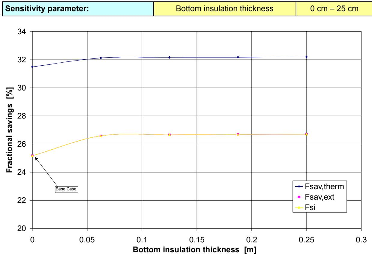
Figure 14. Variation of fractional energy savings with the bottom insulation thickness.
