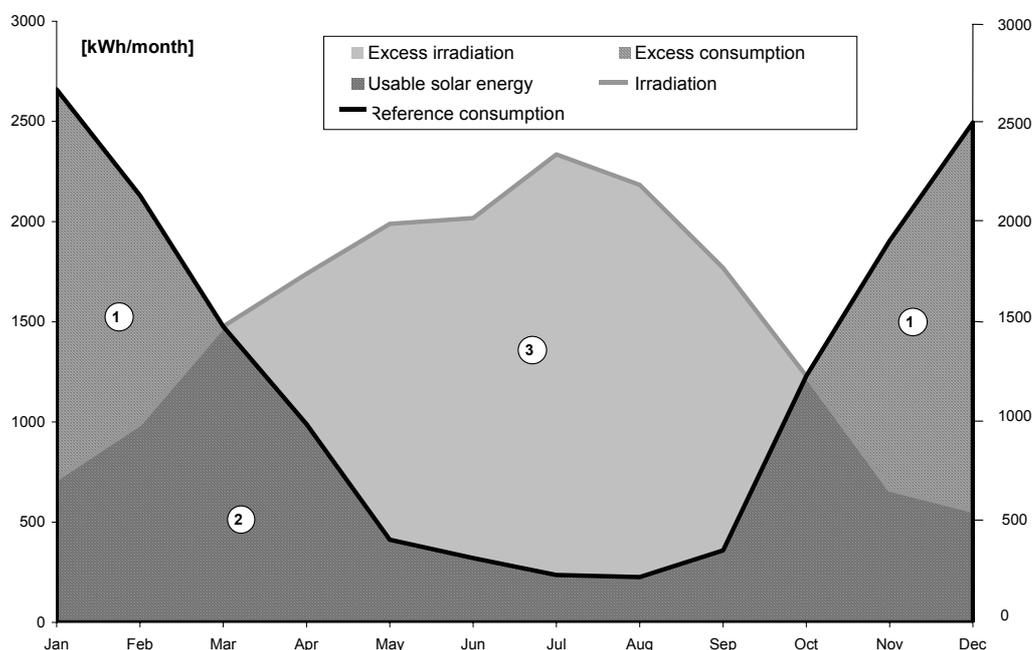
Figure 21: Definition of the fractional solar consumption FSC
