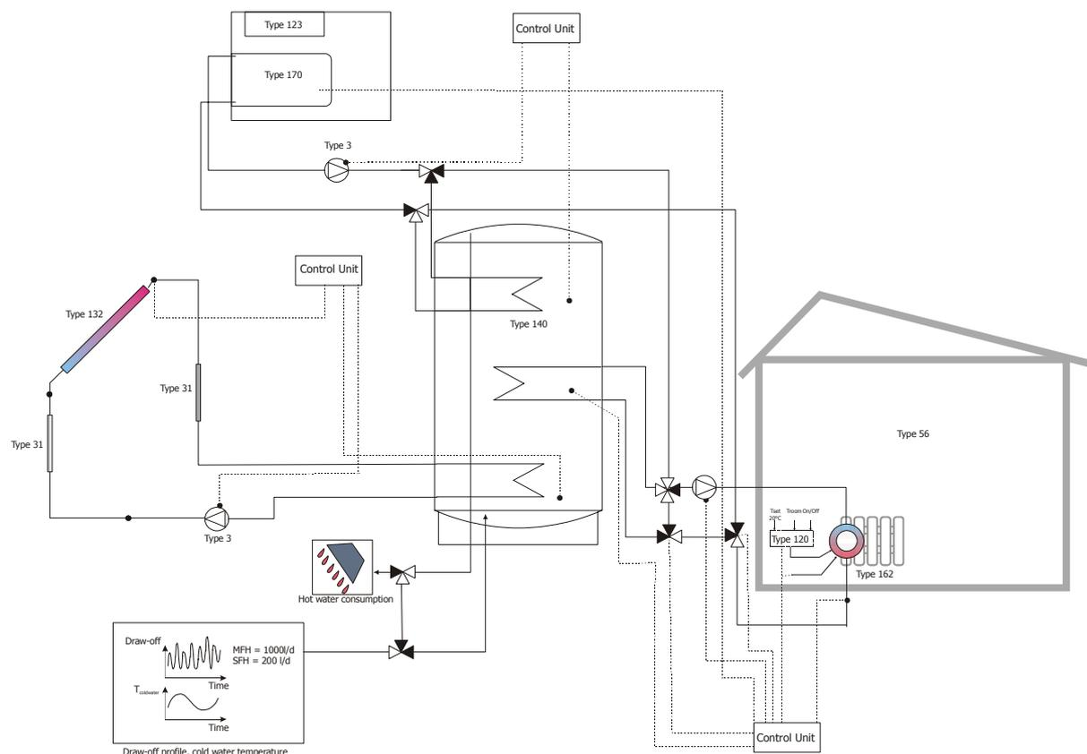
Figure 2: Diagram of System #4 modelled in TRNSYS 14.2.
