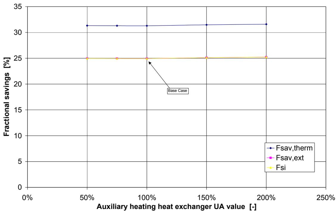
Figure 11. Variation of fractional energy savings with the UA-value of the auxiliary heat exchanger. Parameter values are relative to the base case UA-value.
