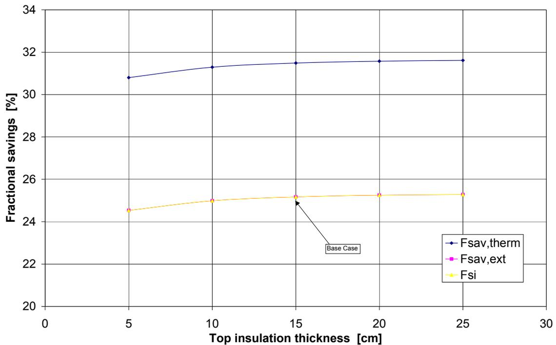
Figure 12. Variation of fractional energy savings with the top insulation thickness.
