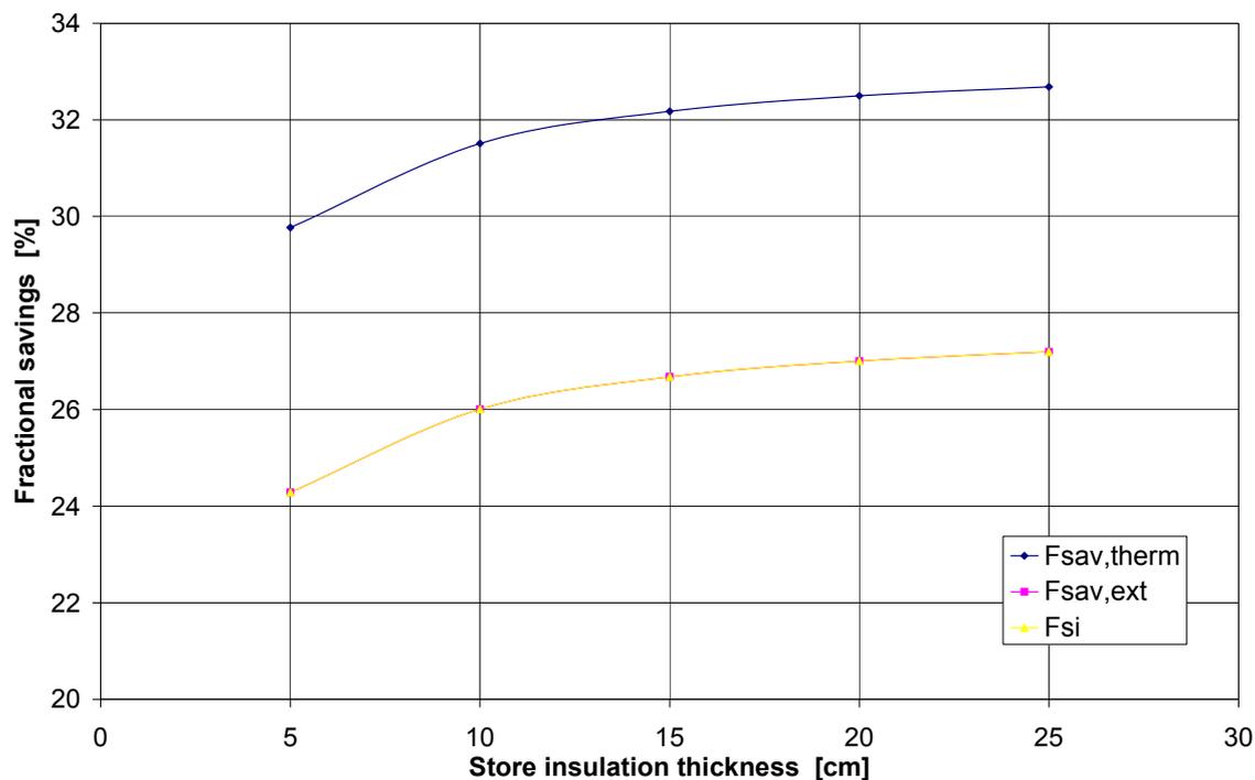
Figure 15. Variation of fractional energy savings with the store insulation thickness.
