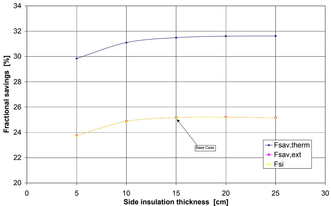
Figure 13. Variation of fractional energy savings with the side insulation thickness.
