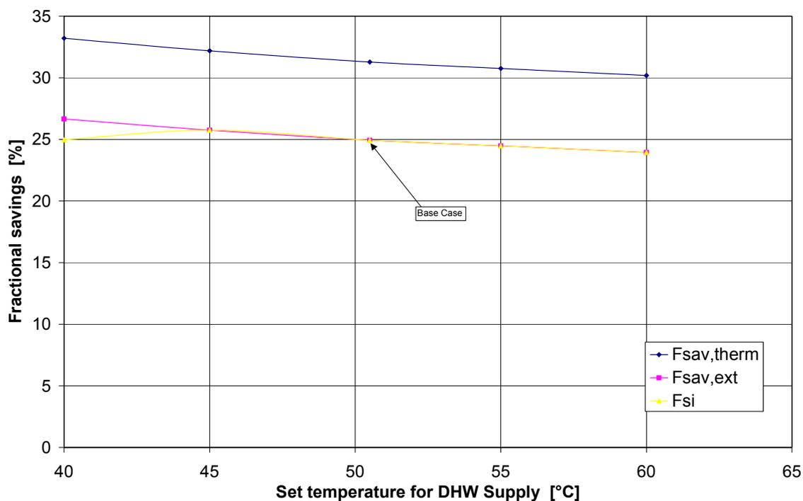
Figure 17. Variation of fractional energy savings set temperature for DHW supply.
