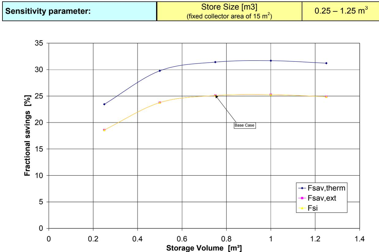
Figure 5. Variation of fractional energy savings with store volume with fixed collector area of 15 [m<sup>2</sup>].
